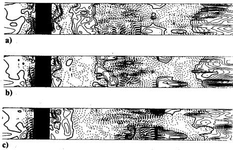
Fig. 9 Regions of instantaneous negative u ; solid, positive; dash, negative; thick solid, 0; increment, 0.016: a) t=0 ; b) t=\Delta t ; and c) t=2\Delta t .
