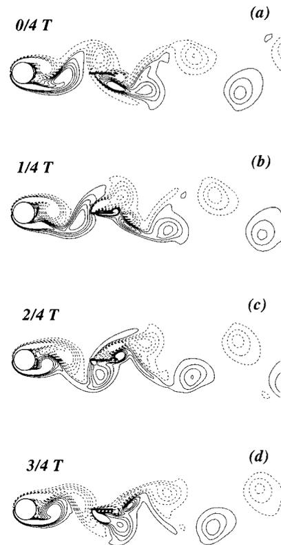
FIG. 7. Instantaneous spanwise vorticity ( $\omega$ ) contours at equal intervals during one period of vortex shedding,  $Re=160$ ,  $G/d=2.7$ . Here,  $T$  is the period of vortex shedding, and  $\Delta\omega d/U_\infty=0.56$ .
