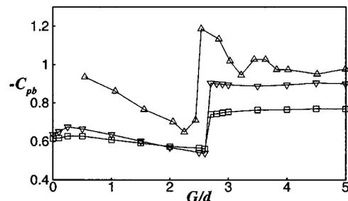
FIG. 4. Variation of the base suction coefficient ( $C_{pb}$ ) with  $G/d$ ; its negative values are plotted for convenience sake.  $Re=100$  ( $\square$ ),  $Re=160$  ( $\nabla$ ). Experimental data of Ozono (Ref. 7) at  $Re=6.7 \times 10^3$  ( $\triangle$ ). The length of the splitter plate is the same as the diameter of the cylinder.
