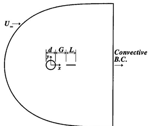
FIG. 1. Schematic diagram of the computational domain.
