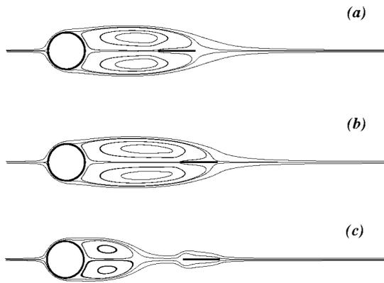
FIG. 5. Time-averaged streamlines for the unsteady flow at  $Re=100$ ; (a)  $G/d=2.0$ , (b)  $G/d=2.6$ , and (c)  $G/d=2.7$ .
