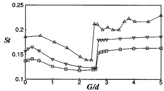
FIG. 3. Variation of Strouhal number ( $St$ ) with  $G/d$ ;  $Re=100$  ( $\square$ ),  $Re=160$  ( $\nabla$ ). Experimental data of Ozono (Ref. 7) at  $Re=6.7 \times 10^3$  ( $\triangle$ ). The length of the splitter plate is the same as the diameter of the cylinder.
