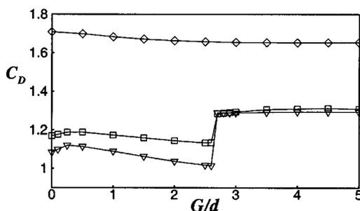
FIG. 2. Variation of drag coefficient ( $C_D$ ) with  $G/d$ ;  $Re=30$  ( $\diamond$ ),  $Re=100$  ( $\square$ ),  $Re=160$  ( $\nabla$ ).
