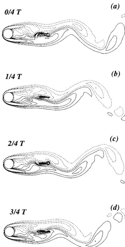
FIG. 6. Instantaneous spanwise vorticity ( $\omega$ ) contours at equal intervals during one period of vortex shedding,  $Re=160$ ,  $G/d=2.6$ . Here,  $T$  is the period of vortex shedding, and  $\Delta\omega d/U_\infty=0.56$ .
